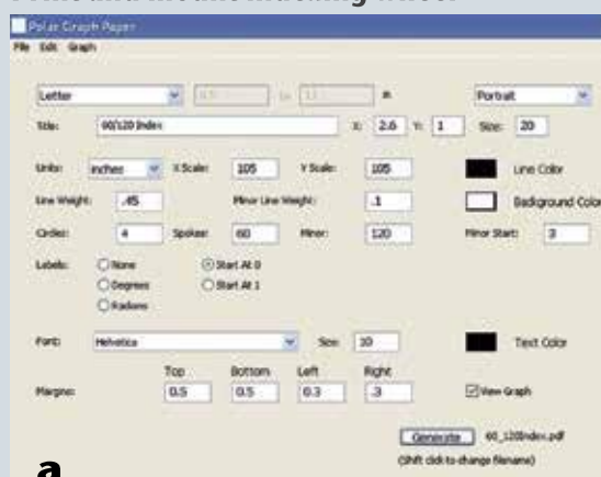
Graph Paper Maker screenshot shows the settings for printing an indexing wheel with 60 and 120 spokes. The printed polar graph is then taped to a hardboard disk and a hole cut out of the center for a completed indexing wheel.
