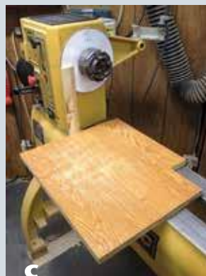
Indexing board in position and anchored to the lathe bed with several rare earth magnets. The top of the vertical riser aligns with the indexing wheel's spokes at the lathe's center height. The pencil jig slides easily on the board's smooth surface.
