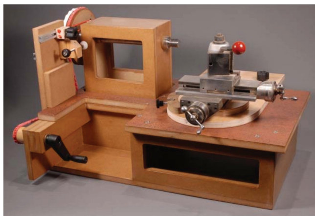
MDF Do-It-Yourself Rose Engine promoted by Jon McGill. This design was published in the American Association of Woodturners Magazine
